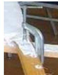
Once square, affix C clamps to center of overlapping bars with screws pointing up
